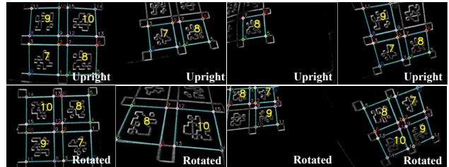
Figure C7. AprilTag detection and corner indexing results for various rotations. Each quad and detected tag ID is colored cyan and yellow, respectively. The unique number for the corner is colored the same as its corner color.
